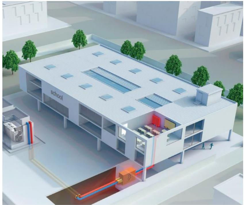
Figure 1. Schematic power substation design next to a school in London
