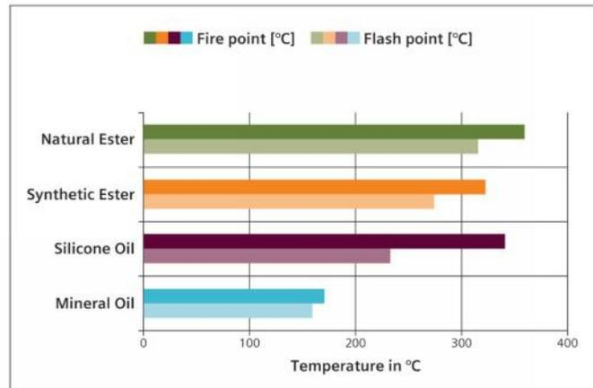
Figure 2. Comparison of the fire and flash points of various insulation oils [1]
